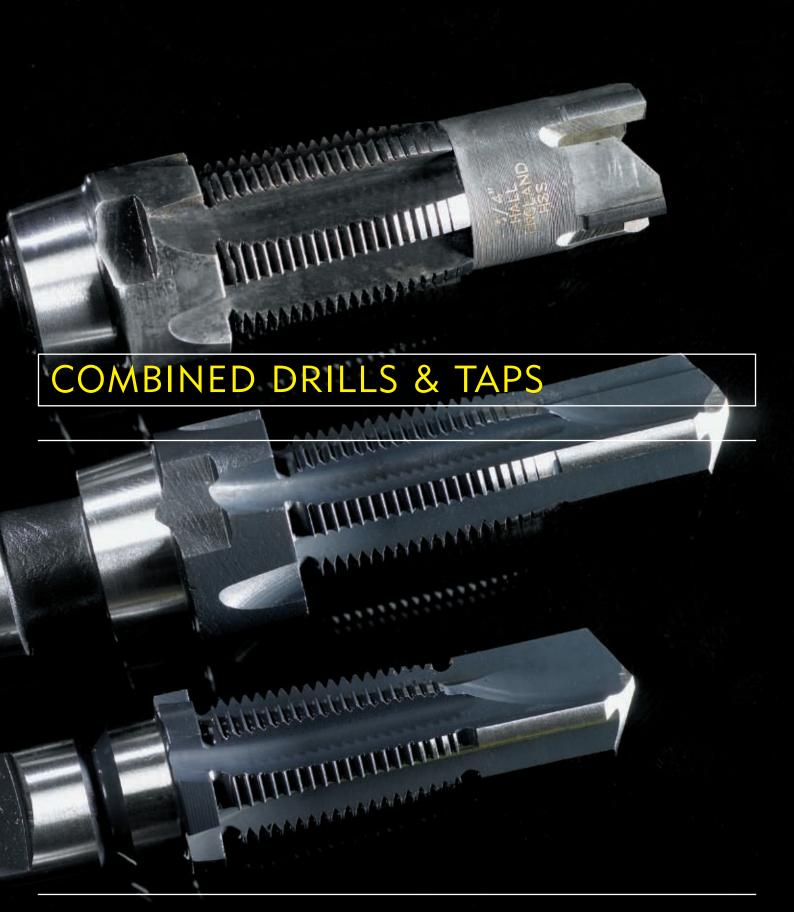
Designed for use during the installation of feed connections etc in gas and water mains. These tools are manufactured from quality carbon chrome tool steel or high speed steel with ground threads and special anti-shock treatment. High speed steel drill taps and cups give better life on cement lined pipes and are usually preferred where the drilling operation is power assisted.
